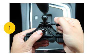
Remove the detachable center blade by rotating the connecting pin until both the dot on the pin and the dot on the mount are facing the same direction, then removing it as shown.
