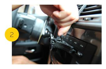
Insert the nGroove blade into your vehicle's CD slot and turn the tightening screw clockwise. The blade will slowly expand. Stop once the nGroove Snap holds securely. The nGroove Snap should not move after installation, but do not overtighten. Failure to comply may cause permanent damage to your stereo.
