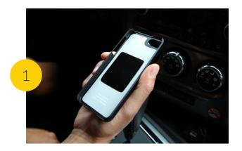
Peel the adhesive protector off of the metal badge and stick it to the back of your device or device case. Note that the badge will also provide a firm hold if you place it between the back of the device and your device case, to hide the badge for a completely invisible look .
