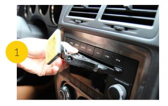
Completely loosen the tightening screw, so the nGroove blade is in a closed position.
