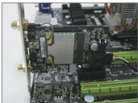
Step 1: Install the Wi-Fi/Bluetooth card in a PCI Express x1 slot. Connect one end of the USB cable to the USB connector on the Wi-Fi/ Bluetooth card.
