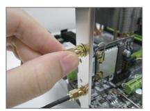
Step 3: Tighten the two antenna cables to the antenna connectors on the Wi-Fi/Bluetooth card respectively.
