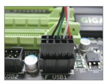
Step 2: Connect the other end of the USB cable to the F\_USB connector on the motherboard.
